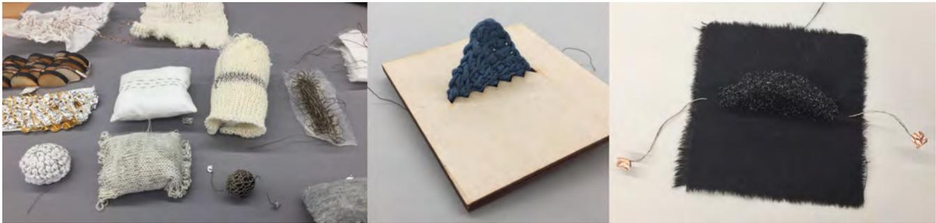
**Figure 1:** Example sensor objects made by designer-author Charlotte Nordmoen. A permanent magnet is typically mounted underneath or inside each object.
