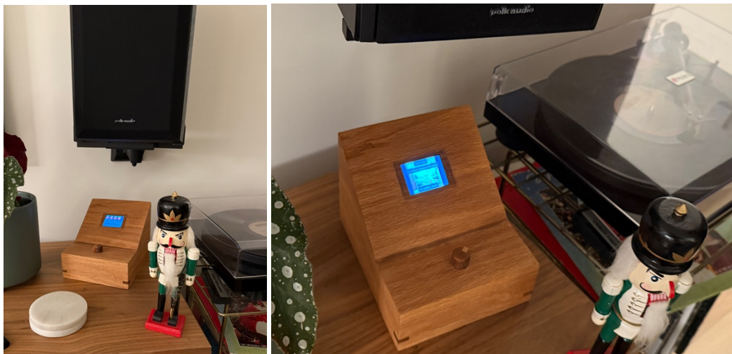
Figure 2. The ‘vinyl scrobber’ handcrafted by P1 composed of mahogany wood, a Raspberry Pi mini computer and display paired with a mobile application for logging vinyl listening histories manually.
